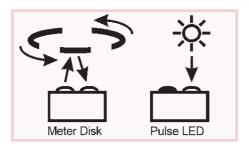
When scanning passive optical indicators (meter disks) the revolutions of the stroboscopic disk are converted into electrical pulses. When scanning active optical indicators (pulse LED) the energy-proportional pulses of electronic counters are registered. The coverage ranges from green, yellow and red LEDs up to IR emitting LEDs.
